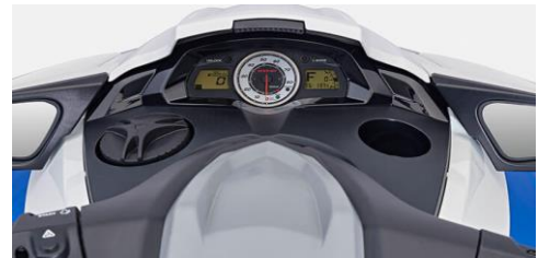
The dash display useful operating functions while Cruiser models also provide air temperature, water temperature, trip Meter, fuel consumption display , and Compass
