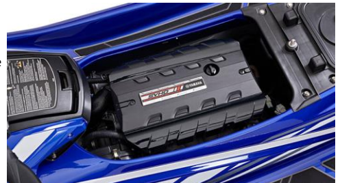
Yamaha's 1.8L supercharged, Super Vortex High Output Marine engine delivers more power and torque than any WaveRunner Personal WaterCraft before it
